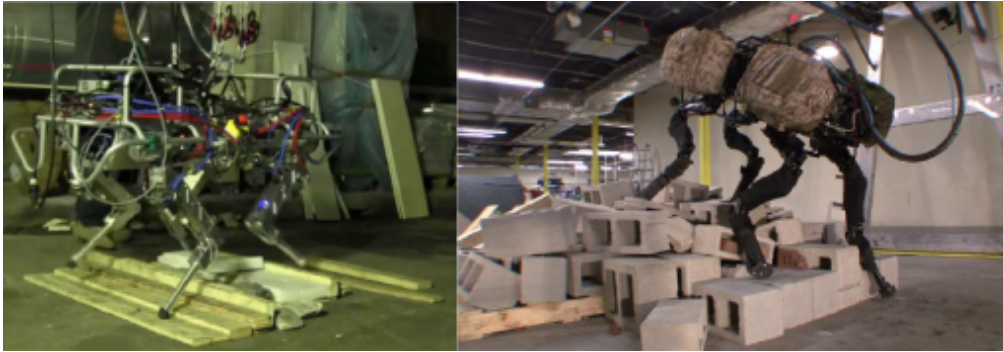
Figure 1.11: HyQ balancing on rough terrain [Barasuol et al., 2013] and Big Dog descending on rubble [Raibert et al., 2008]
