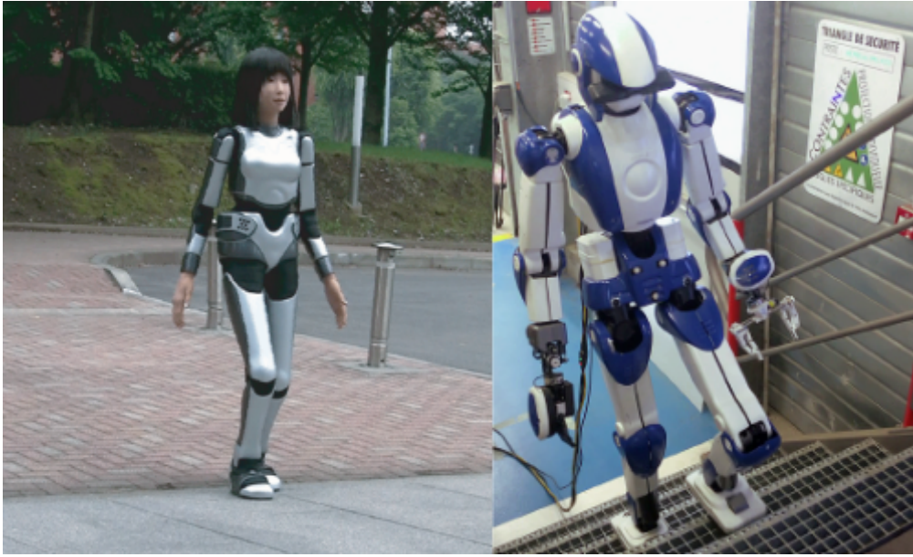
Figure 1.14: HRP-4 Walking on Pavement (left) [Kajita et al., 2010] and Climbing Stairs (right) [Caron et al., 2021]
