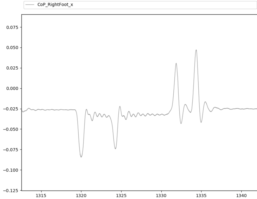
Figure 5.17: CoP of the RF of HRP2-KAI on rigid floor while resisting pushes
