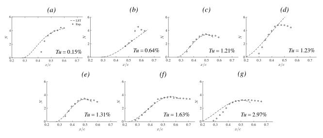
Figure 7 – Comparison of experimental (markers) LST (dashed line) predicted N–factors for frequencies within the excitation bands from Fig. 3 for configurations where a laminar separation bubble is present. Initial disturbance amplitudes are estimated through matching LST and experimental N–factors
