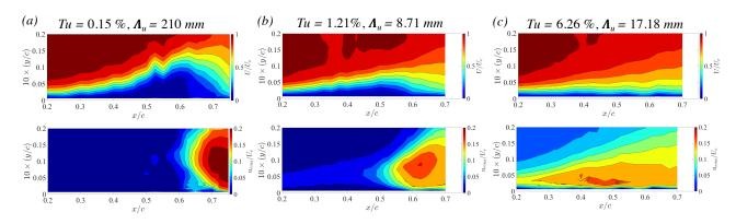
Figure 2 – Contours of the mean streamwise velocity (U) and the r.m.s of the fluctuating streamwise velocity ( $u_{rms}$ ) (a) 0.15% (b) 1.21% and (c) 6.28%.
