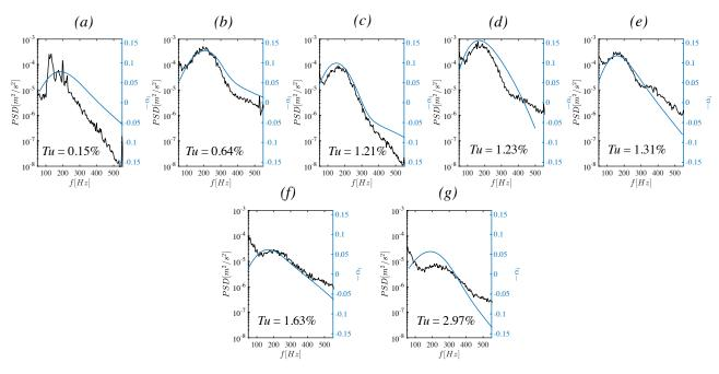
Figure 5 – Comparison between the amplified frequencies predicted by LST to the experimental spectra. NB: Two different y-axes for  $\alpha_i$  and the power from the PSD, therefore direct comparisons between the two are not be made.
