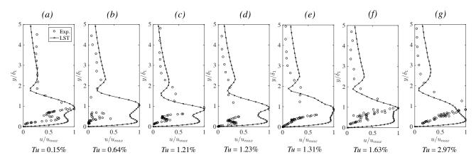
Figure 6 – Experimental filtered disturbance profiles in the wall-normal direction compared to the eigenfunction for the most amplified frequency from LST. Experimental streamwise disturbance profiles are computed by applying a bandpass filter corresponding to the lost amplified frequency band from the PSD.
