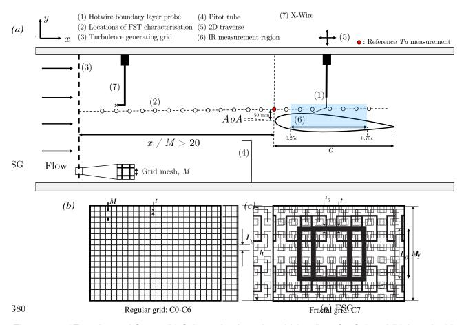
Figure 1 – a )Experimental Setup. (b) Schematic of regular grid (configs. C0-C6) and (b) fractal grid (config. C7)
