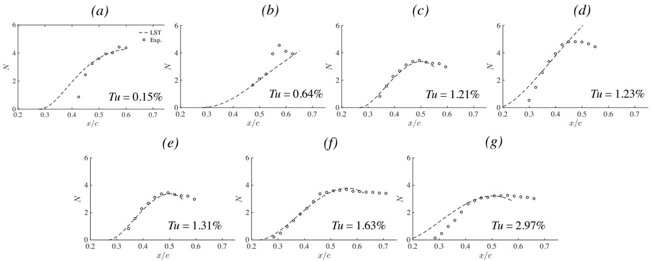
Figure 7 – Comparison of experimental (markers) LST (dashed line) predicted  $N$ -factors for frequencies within the excitation bands from Fig. 3 for configurations where a laminar separation bubble is present. Initial disturbance amplitudes are estimated through matching LST and experimental  $N$ -factors
