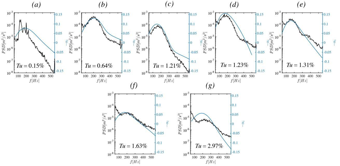
Figure 5 – Comparison between the amplified frequencies predicted by LST to the experimental spectra. NB: Two different y–axes for  $\alpha_i$  and the power from the PSD, therefore direct comparisons between the two are not be made.
