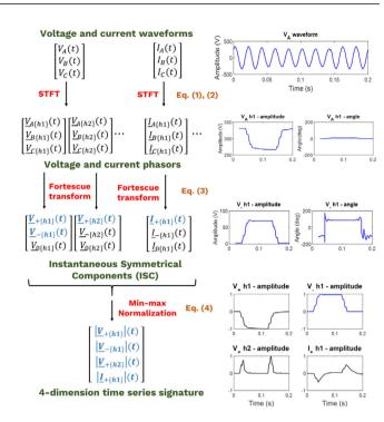
**FIGURE 3** Detailed steps of the pre-processing and obtained components for the calculation of the four-dimensional signatures
