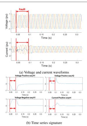
FIGURE 4 Voltage sag caused by an upstream non-symmetrical fault (real measurement data)
