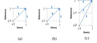
FIGURE 7 Local step patterns: (a) symmetric1, (b) symmetric2, (c) asymmetric [44]
