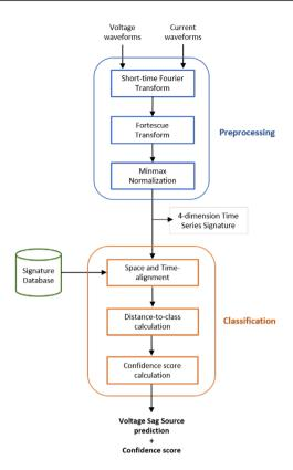
FIGURE 2 Flowchart of the proposed voltage sag source classification method
