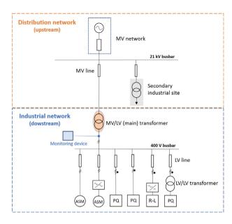
FIGURE 1 Simplified diagram of the industrial network model
