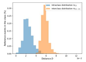
**FIGURE 11** Intra-class distribution  $\mathcal{H}_{C2}$  and inter-class distribution  $\mathcal{H}_{C2-C1}$ , with BC=0.07
