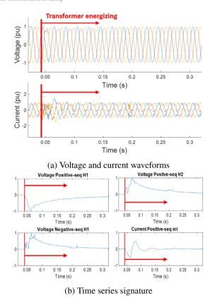
FIGURE 5 Voltage sag caused by an upstream transformer energizing (real measurement data)
