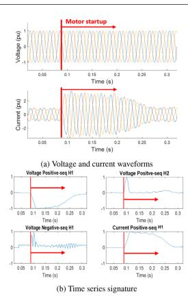
FIGURE 6 Voltage sag caused by a downstream induction motor startup (real measurement data)
