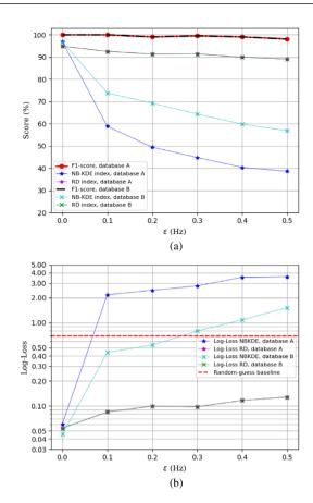
**FIGURE 13** F1-score and mean values for NB-KDE and RD indexes (a) and the corresponding Log-loss values (b) associated to the classification outputs, for different levels of fundamental frequency variations,  $F=50~{\rm Hz}$
