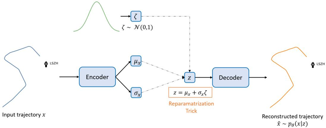
Figure 3: Basic architecture of a Variational Autoencoder
