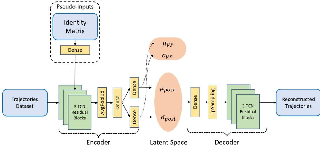
Figure 5: Structure of the proposed VampPrior TCVAE.  $\mu_{VP}, \sigma_{VP}$  stand for the VampPrior parameters, and  $\mu_{post}, \sigma_{post}$  for the ones of the posteriors.
