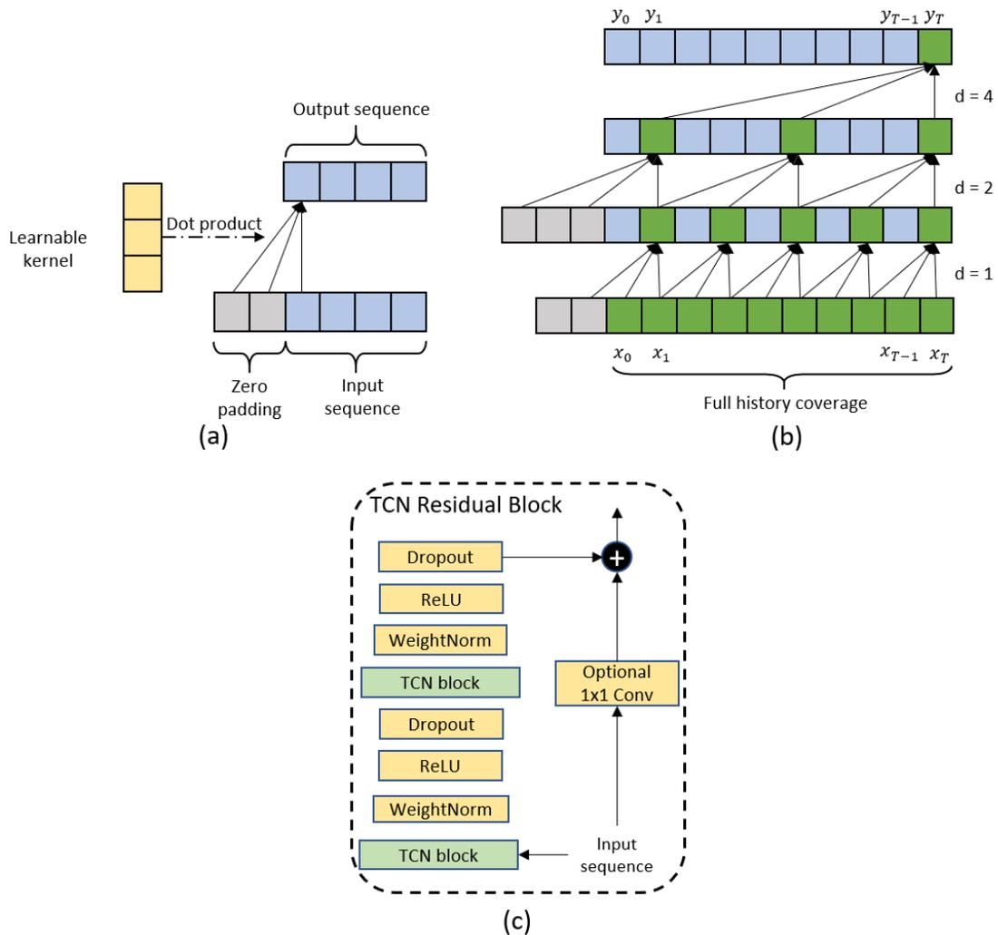
Figure 4: Architectural elements of a TCN. (a) represents a 1-dimensional convolutional layer with a kernel size of 3. (b) represents 4 1-dimensional convolutional layers with a kernel size of 3 and a dilatation factor of 2, called a TCN block. (c) represents the full structure of a TCN residual block, which is the base architectural element of a TCN.
