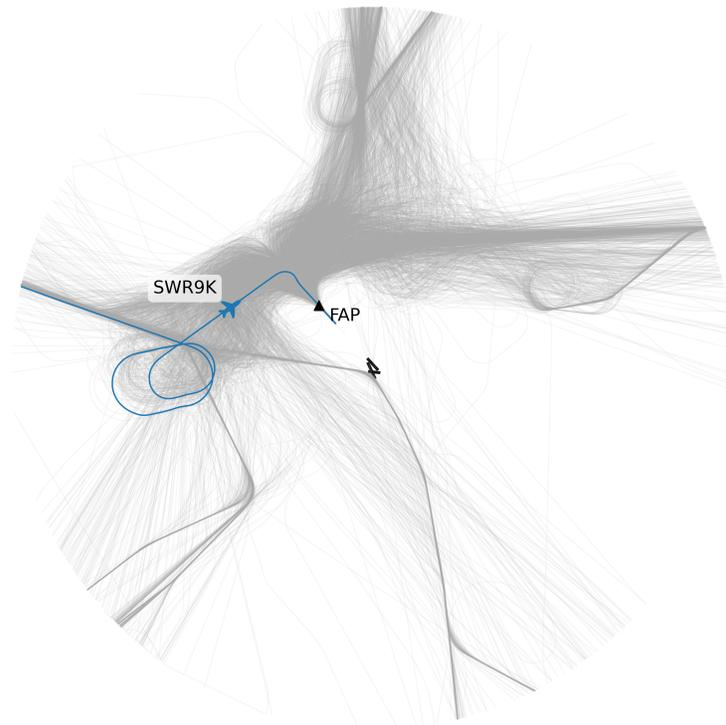
Figure 2: Historical landing trajectories downloaded with OpenSky Network between 1st October and 30 November at Zurich Airport for runway 14
