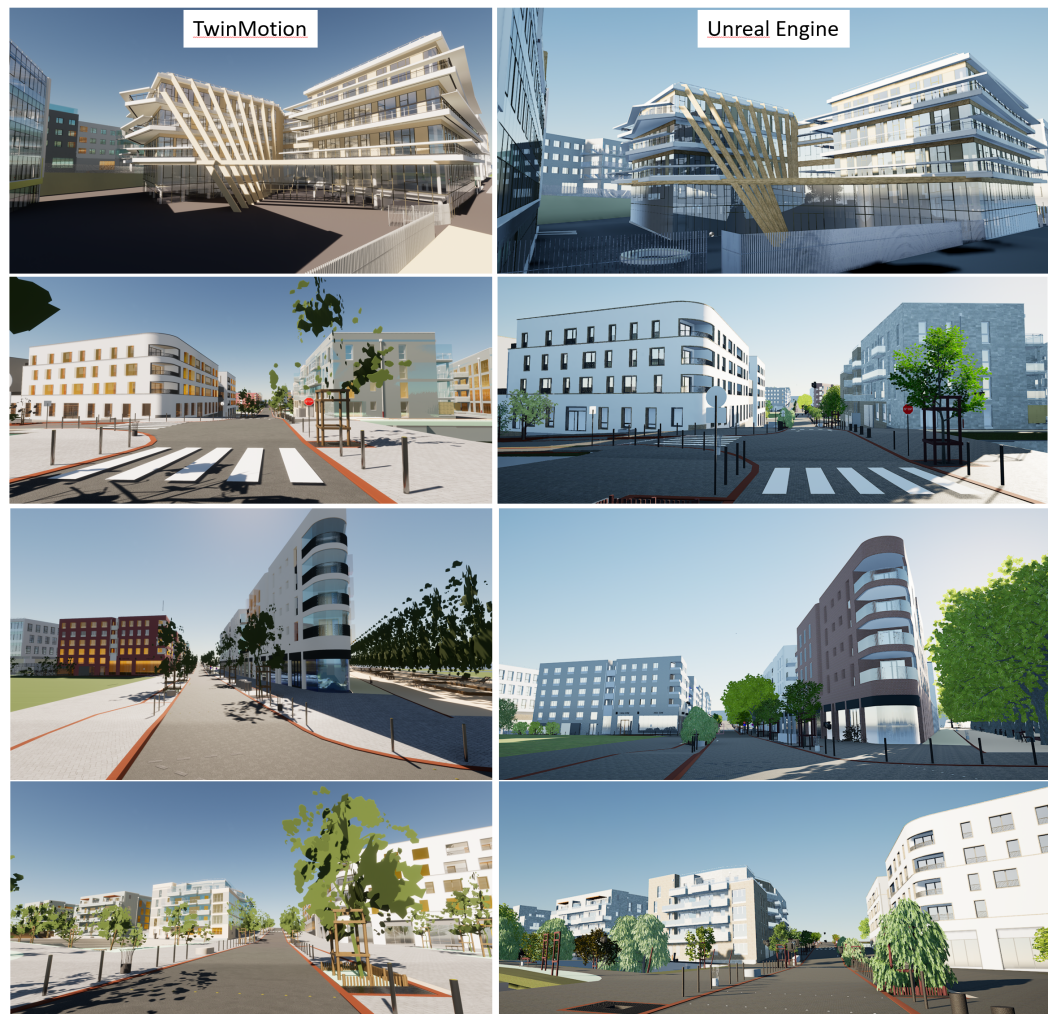
Figure 19. Left: TwinMotion project. Right: Unreal Engine scene. The Unreal Engine texture and lighting conform more to reality than the TwinMotion scene, which is more cartoonish.
