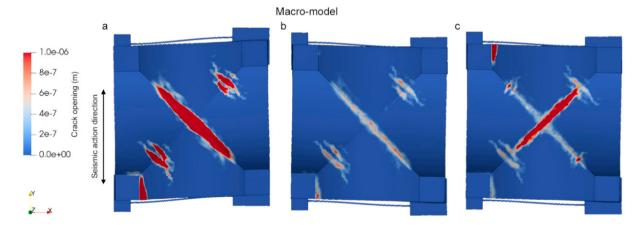
Fig. 5. Reclosure of the crack opening for the macro-model at a) 3.4 s, b) 3.7 s and c) 3.8 s of the seismic input applied in the nonlinear dynamic analyses performed (top view).
