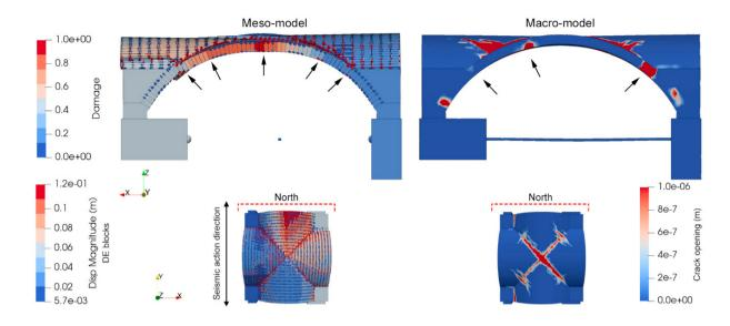
Fig. 4. Comparison of the cross vault numerical damages of the meso- and macro-model from the North view.
