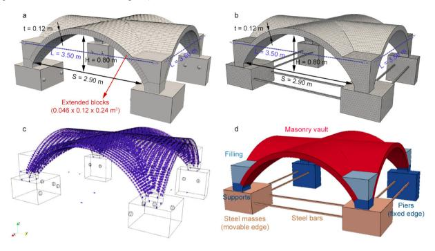
Fig. 2. Geometry of the numerical a) discrete and b) continuum models. Detailed views of c) the contacts in the discrete approach and d) a scheme of the materials adopted in both modeling strategies.
