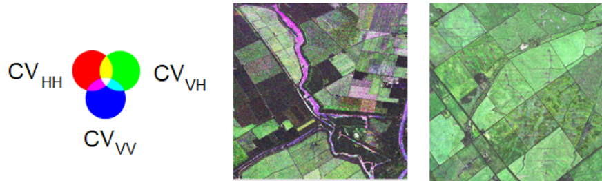
Figure 3: Composition of the different coefficient of variations obtained in HH, VV and VH polarization - UAVSAR -
