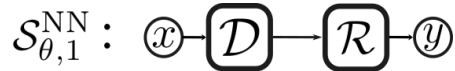
FIGURE 2. Definition of \mathcal{S}_{\theta, 1}^{NN} where \mathcal{D} represents a convolution neuron (or diffusion neuron in reference to diffusion operators), and \mathcal{R} represents a multilayer perceptron (called reaction network in reference to reaction operators). The parameter \theta is the vector of learning parameters, it contains all weights of the \mathcal{D} and \mathcal{R} networks.
