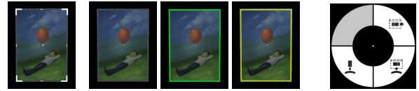
Figure 3: Visual feedback on the CARDS and menus. On the left: a corner highlight added in AR when the user gazes at the CARD (not seen by others). In the middle, the CARD selection states, visible by all users: the CARD in its unselected state; the CARD selected by a user who is assigned the green color; and by the user who is assigned yellow. The last image shows our contextual menu, only visible to the user that invokes it. In this case, the contextual menu has been invoked on a CARD that exists on a virtual surface, so we see the available options to move all content of the surface towards another surface (top-right) or the Personal Space (bottom-right), or to move the CARD to the Personal Space (bottom-left).
