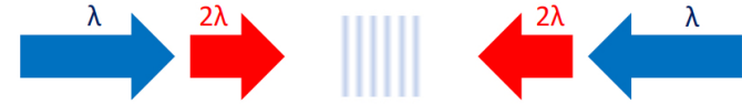
Figure 6. The principle of a superlattice: two standing light waves are superimposed, the first one with wavelength \lambda and the second one with wavelength 2\lambda .
