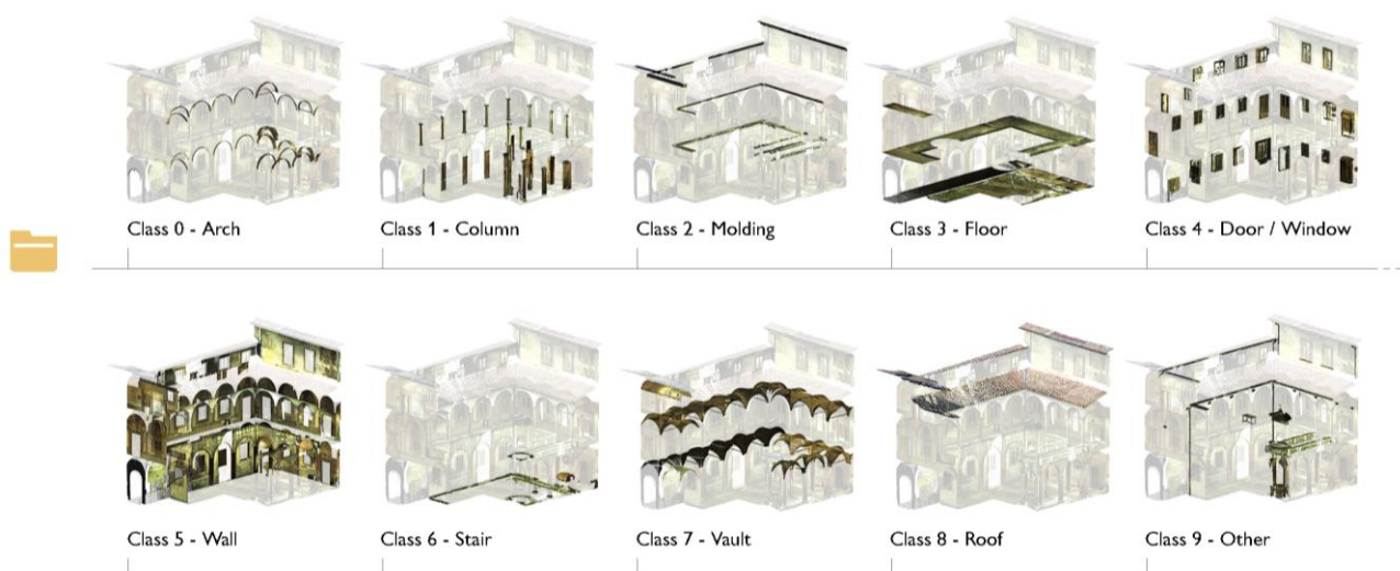
Figure 12. Two isolated classes of architectural components from the initial point cloud using example from the Grand-Ducal cloister, Pisa Charterhouse.
