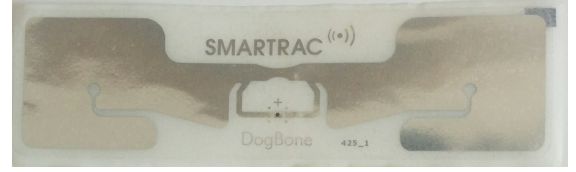
Fig. 5. Smartrac Dogbone UHF RFID tag with Impinj chip.
