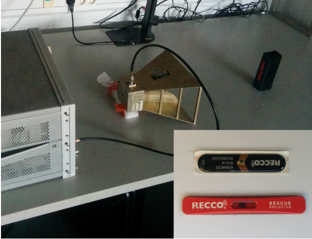
Figure 2. Measurement bench used in the study. Inset: Harmonic transponders (RECCO reflectors).
