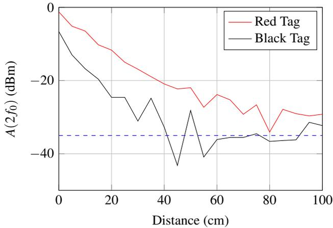
**Figure 5.** Read range associated to the presented harmonic transponders at 915 MHz.
