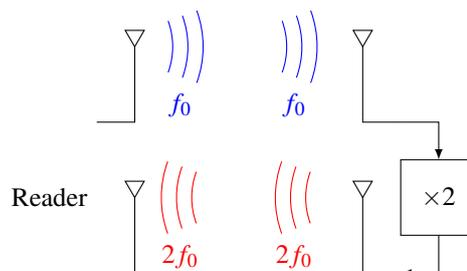
Figure 1. Principle of the harmonic reading system.
