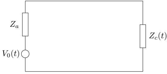
Fig. 1. Equivalent circuit of a minimum scattering antenna with open circuit voltage V_0(t) and loaded by a RFID chip Z_c(t) excited by a modulated signal.
