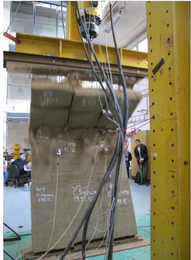
Fig.5: Final collapse of testing 1.8 x 3.0 x 0.2 m wall consisted of 10 prefabricated rammed earth panels. Load bearing capacity 16N/mm 2 , final vertical deformation 1.2% (37 mm).
