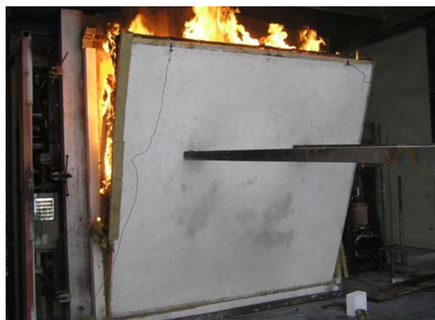
Fig 6: Test of 3x3 m load bearing straw bale wall specimen with clay plaster from interior in fire chamber at the end of the experiment. Final result: fire resistance REI 120 min (2h26')
