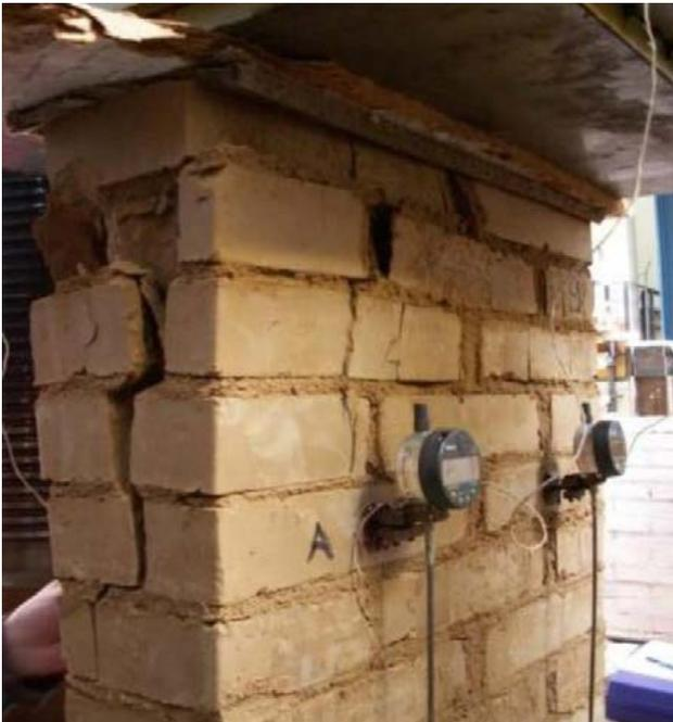
Fig.4: 600/150/900mm pillar failure cracks at mid-width and mid-thickness accompanied by other faults. Various wall sizes, clay materials, walls bonding pattern and the influence of moisture content were tested during the research.
