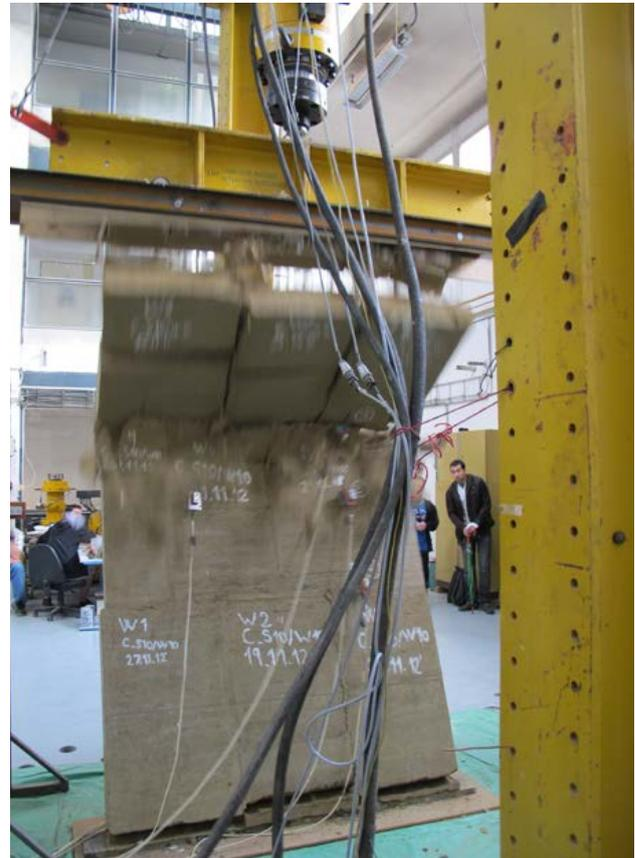
Fig.5: Final collapse of testing 1.8 x 3.0 x 0.2 m wall consisted of 10 prefabricated rammed earth panels. Load bearing capacity 16N/mm<sup>2</sup>, final vertical deformation 1.2% (37 mm).
