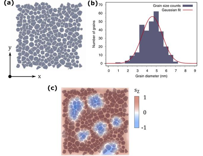
FIG. 2. (a) The bare grain structure of the AFM layer created using a Voronoi construction. (b) The grain size distribution showing an average grain size of  $\sim 4.5 \text{ nm}$ . (c) Overlaying the FM layer spin structure and the bare grain structure shows that the irregular shape of the skyrmions in the former follows the grain boundaries of the latter.
