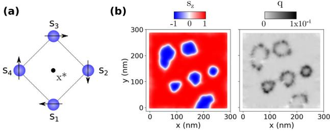
FIG. 6. (a) Schematic showing the method for calculating the topological charge density  $q$  of a discrete lattice made up of square unit cells. The total topological charge  $Q$  is the sum of  $q$  over the entire lattice. (b) The topological charge density calculated for the FM layer.
