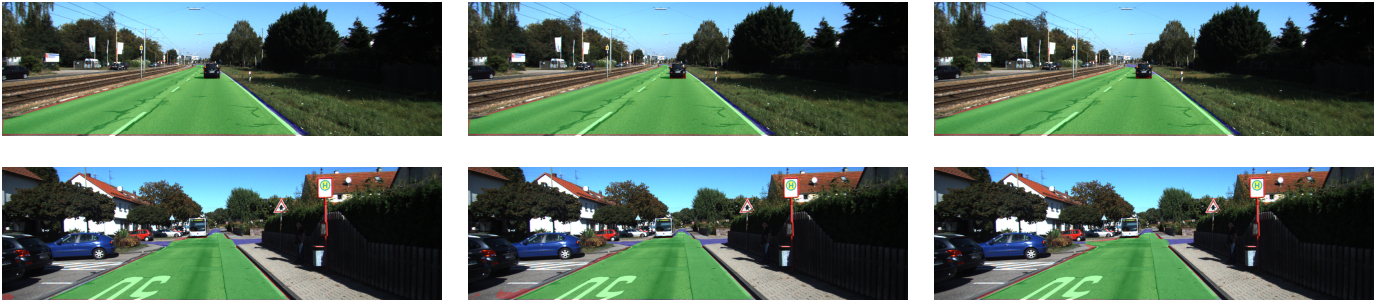
Fig. 4: Detection output of the baseline and reduced architectures. From left to right: baseline prediction, uni-decoder CF prediction, Lite CF prediction [Green: True positive, Red: False positive, Blue: False negative].
