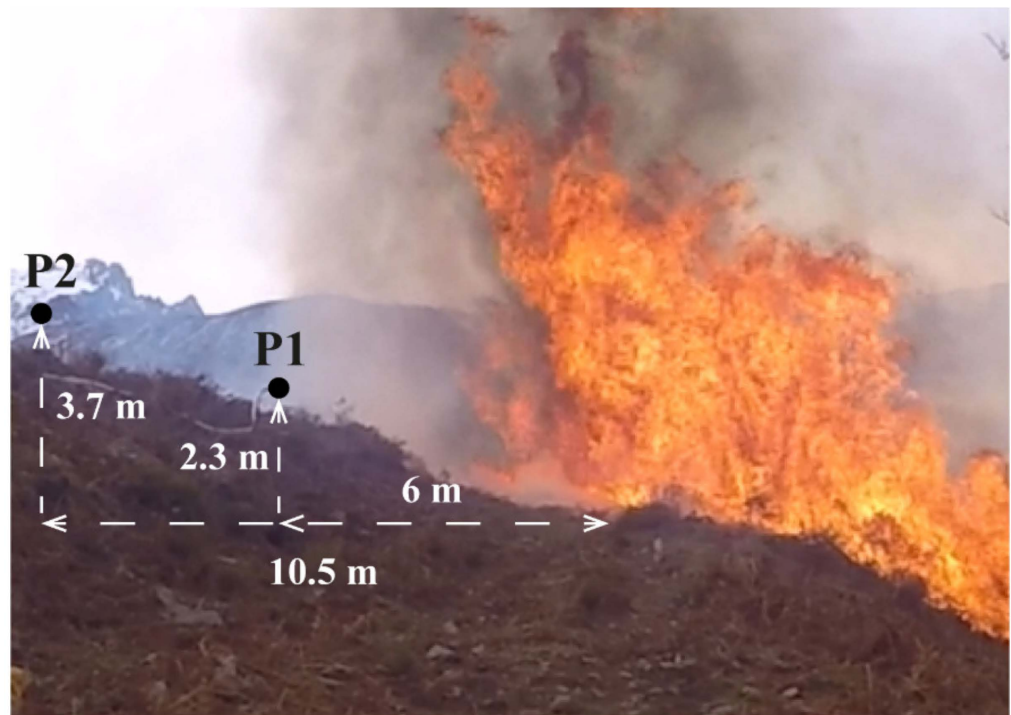
Figure 11. Positions P1 and P2 of the radiant and total fluxmeters with respect to the plot end (March 2022 experiment).
