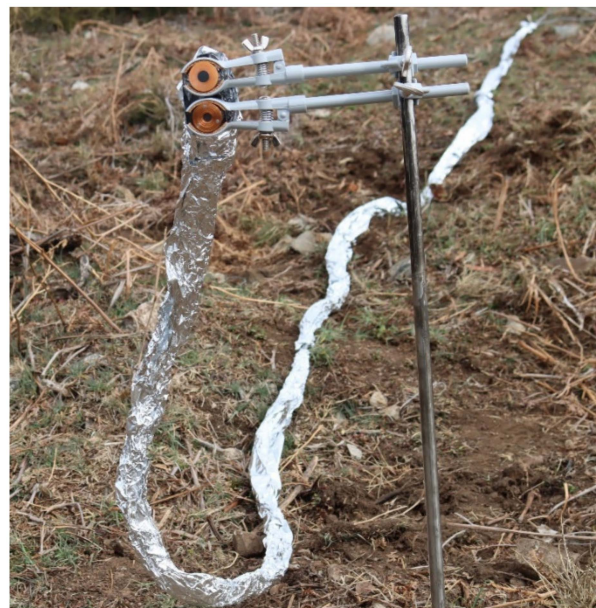
Figure 3. Radiant and total heat flux sensors fixed on supporting rod ahead of the vegetation plot and protected with aluminum foil.
