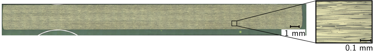
Figure 1: Micrograph (cross section parallel to the fibers main axis) of the consolidated samples before deconsolidation tests. The initial porosity content is not measurable.
