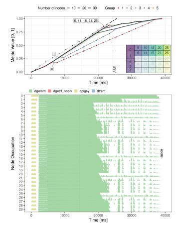
Fig. 6. Progression visualization strategy and aggregated Gantt chart of Chameleon's LU Factorization simulation over 30 nodes where the first and second nodes received 50% and 25% more load, respectively.
