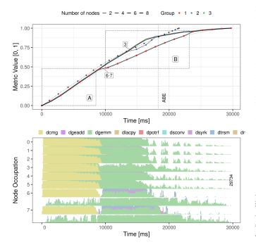
Fig. 8. Progression visualization strategy (with a bandwidth of 0.15) and aggregated Gantt chart of ExaGeoStat real execution iteration on eight heterogeneous nodes.
