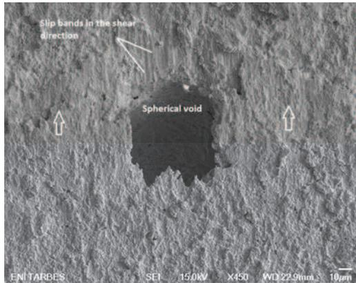
**Figure 2: Micrographs of AuGe specimen failure profiles: initial voids fraction due to reflow process.**
