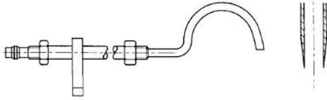
Figure 3: Suction iso-kinetic probe.
