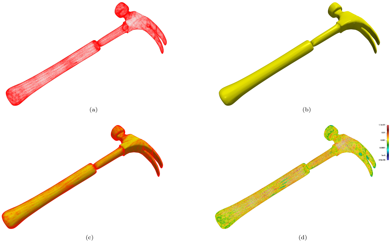
Figure 13: Hammer. (a): point cloud obtained sampling an ACC surface. (b): final least square surface. (c): comparison between point cloud and final surface. (d): colorplot of the \ell_2 distances contained in \mathbf{err} in logarithmic scale.
