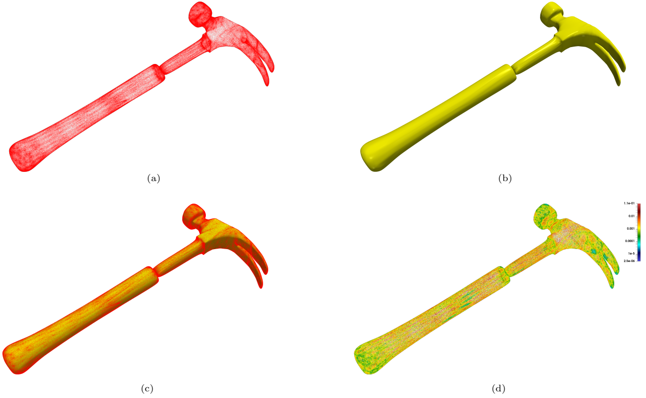
Figure 13: Hammer. (a): point cloud obtained sampling an ACC surface. (b): final least square surface. (c): comparison between point cloud and final surface. (d): colorplot of the \ell_2 distances contained in err in logarithmic scale.
