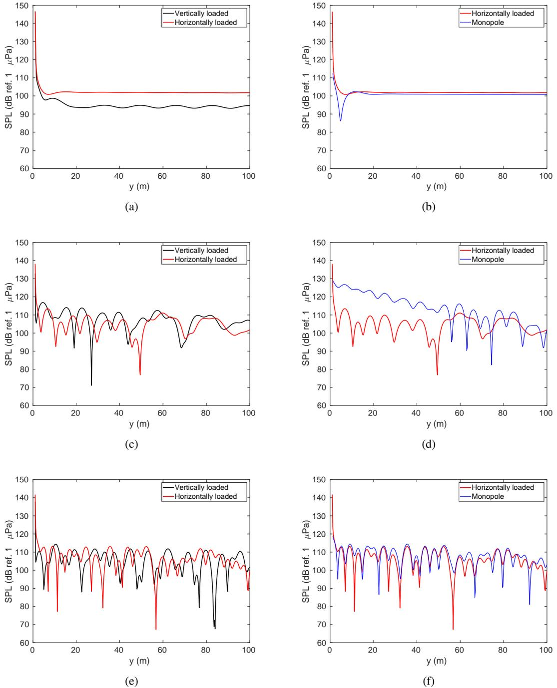
**Figure 13:** Acoustic sound pressure along  $(x = 0, y)$  for a vertically loaded shell, horizontally loaded shell and pulsating monopole positioned at the midpoint of a shallow waveguide with total depth  $H = 10$  m. Comparison between a vertically loaded shell and horizontally loaded shell (Left) and, between a horizontally loaded shell and pulsating monopole (Right) is shown for the following frequencies: 100 Hz (a,b), 262.5 Hz (c,d), and 500 Hz (e,f).
