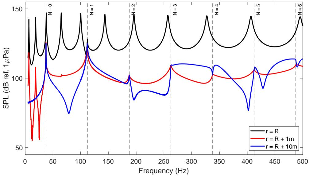
**Figure 8:** Acoustic pressure spectra for a vertically-loaded shell positioned at the midpoint of a waveguide of depth  $H = 10$  m. The observation point is chosen at several locations including: at the surface of the shell ( $r = R, \varphi = \pi/2$ ), 1m from the surface ( $r = R + 1$  m,  $\varphi = \pi/2$ ), and 10m from the surface ( $r = R + 10$  m,  $\varphi = \pi/2$ ).
