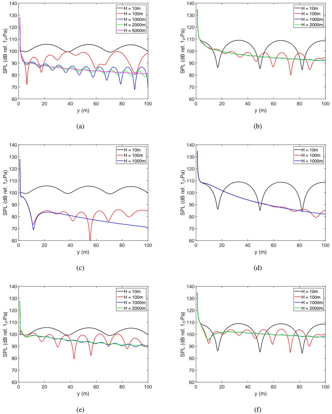
**Figure 15:** Convergence of (a,c,e) vertically loaded shell and (b,d,f) horizontally loaded shell for different waveguide configurations: (a,b) increasing and equally distant from the free surface and seabed, (c,d) with increasing distances of the free surface, and (e,f) with increasing distances of the seabed and at 150 Hz.
