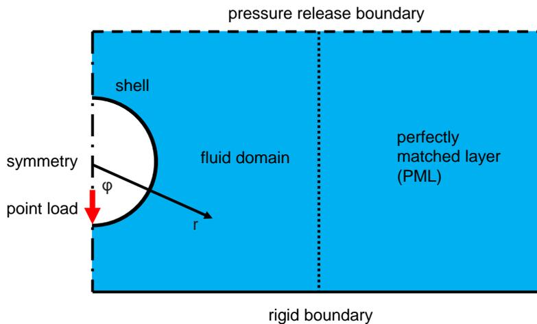
Figure 3: Schematic of the finite element model.
