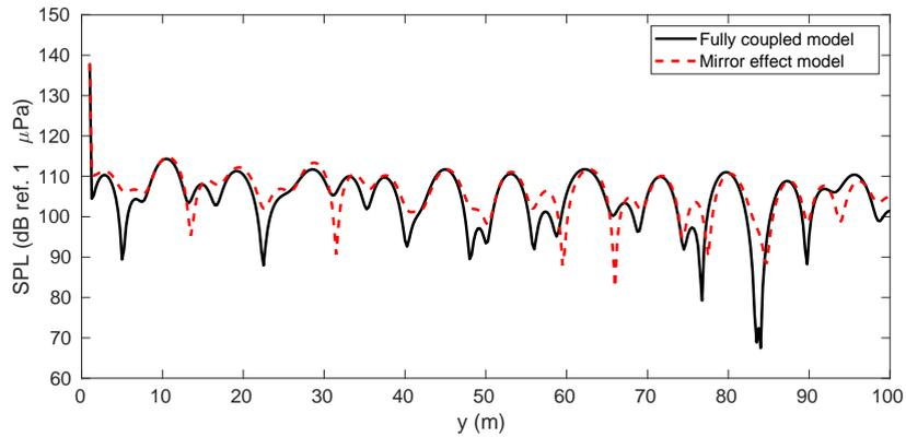
(c) 500 Hz (higher frequency, non-standing wave frequency)
