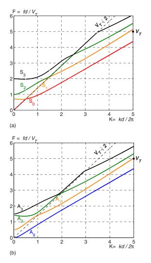
FIG. 4. (Color online) Special behavior at  $\nu=0$  (rigid solid). (a) Symmetric Lamb modes: segments of the Lamé line belong to successive modes. The change from mode  $S_n$  to mode  $S_{n+1}$  occurs at the coincidence point of abscissa K=n+1/2 and gives rise to a discontinuity of the slope. (b) This discontinuous behavior is not observed on anti-symmetric branches.
