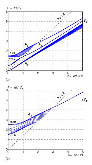
FIG. 1. (Color online) Variation, with Poisson's ratio in the range  $0 \le \nu \le 0.49$ , of anti-symmetric Lamb modes in an isotropic free plate of thickness *d*. Bundle of dispersion curves for (a)  $A_0$ ,  $A_1$ , and  $A_2$  modes, and (b)  $A_3$  mode. For each mode, the lower curve corresponds to  $\nu=0$  and the upper one to  $\nu=0.49$ .
