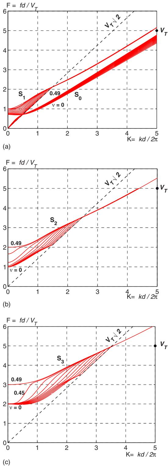
FIG. 2. (Color online) Variation, with Poisson's ratio in the range  $0 \leq \nu \leq 0.49$ , of symmetric Lamb modes in an isotropic free plate of thickness  $d$ . Bundle of dispersion curves for (a)  $S_0$  and  $S_1$  modes, (b)  $S_2$  mode, and (c)  $S_3$  mode. For each mode, the lower curve corresponds to  $\nu=0$  and the upper one to  $\nu=0.49$ .
