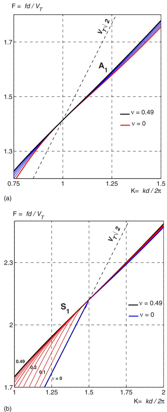
FIG. 3. (Color online) Behavior of dispersion curves over the coincidence points. (a)  $A_1$  mode and (b)  $S_1$  mode. Dispersion curves of a given mode cross the line  $F = \sqrt{2}K$  with the same slope.
