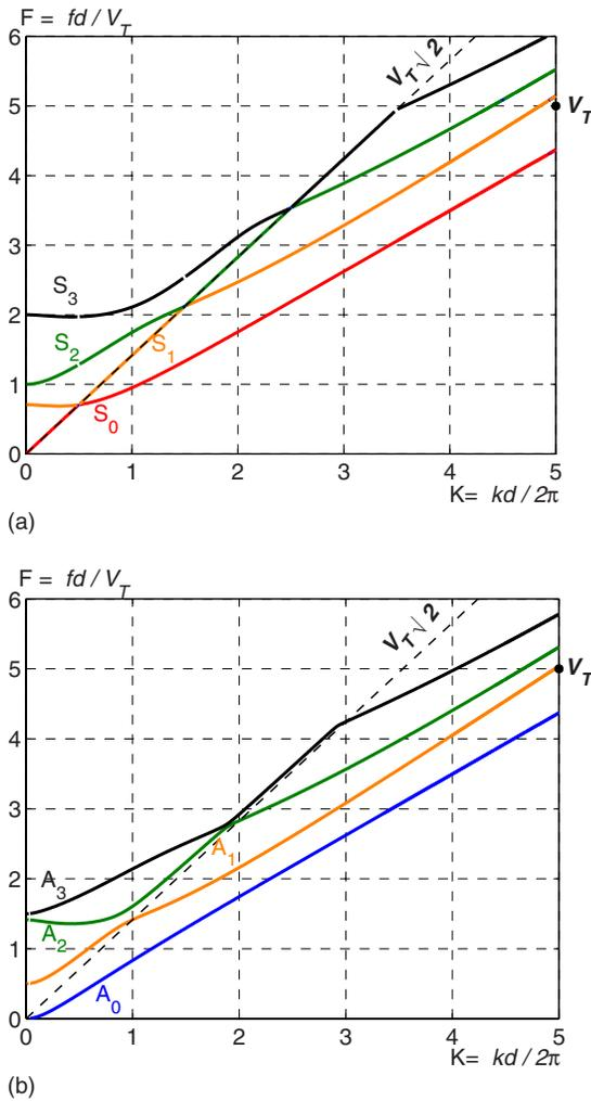
FIG. 4. (Color online) Special behavior at  $\nu=0$  (rigid solid). (a) Symmetric Lamb modes: segments of the Lamé line belong to successive modes. The change from mode  $S_n$  to mode  $S_{n+1}$  occurs at the coincidence point of abscissa  $K=n+1/2$  and gives rise to a discontinuity of the slope. (b) This discontinuous behavior is not observed on anti-symmetric branches.
