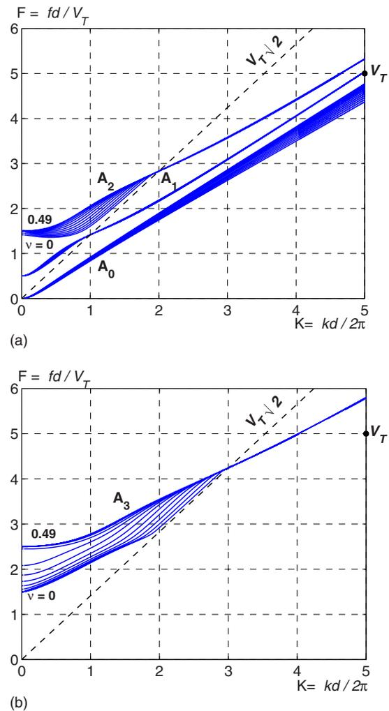
FIG. 1. (Color online) Variation, with Poisson's ratio in the range  $0 \leq \nu \leq 0.49$ , of anti-symmetric Lamb modes in an isotropic free plate of thickness  $d$ . Bundle of dispersion curves for (a)  $A_0$ ,  $A_1$ , and  $A_2$  modes, and (b)  $A_3$  mode. For each mode, the lower curve corresponds to  $\nu=0$  and the upper one to  $\nu=0.49$ .
