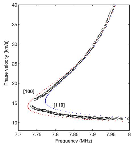
FIG. 8. (Color online) For a line source perpendicular to the  $22.5^\circ$  direction, experimental data (circles) lie in between the curves computed for the  $S_1$  Lamb mode propagating along [100]- and [110]-directions.
