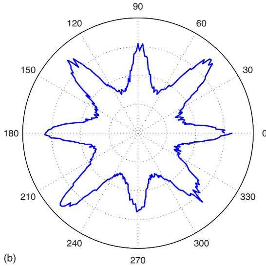
FIG. 3. (Color online) Line laser source. (a) *B*-scan of the spectrum measured as a function of the line orientation. The thickness resonance frequency is constant while the ZGV resonance frequency oscillates with a 90° period. (b) Polar plot (linear scale) of the resonance amplitude versus the propagation direction.
