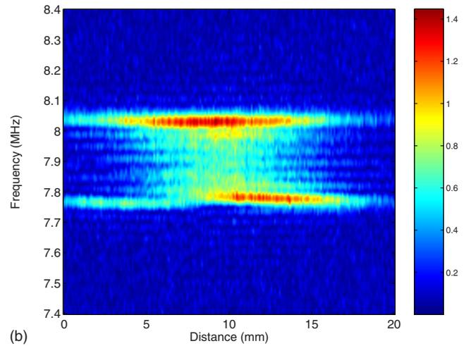
FIG. 5. (Color online) *B*-scan of the resonance amplitude measured along a line parallel to the source at a distance equal to 10 mm. (a) Line perpendicular to the direction  $\varphi=0^\circ$ . (b)  $\varphi=22.5^\circ$ : the energy distribution of the ZGV resonance is shifted from that of the thickness resonance mode.
