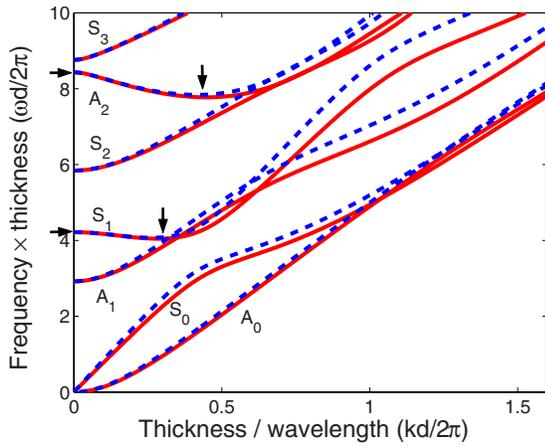
FIG. 1. (Color online) Dispersion curves in the  $(\omega, k)$ -plane for Lamb waves propagating in a silicon plate of thickness  $d$  along the  $[100]$  axis (solid lines) and the  $[110]$  axis (dashed lines). Vertical arrows correspond to ZGV modes, and horizontal ones to thickness resonance frequencies.
