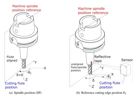
Figure 5: Identification of reference flute position
