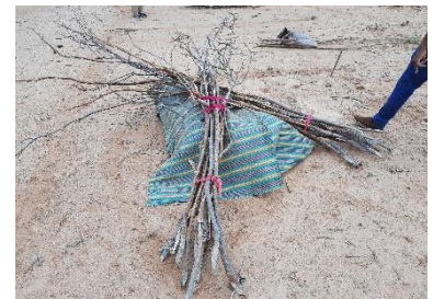
Branches necessary for the construction of a buul . Doolow, Jubaland – CC Enrique Sevillano Gutiérrez, CRAterre
