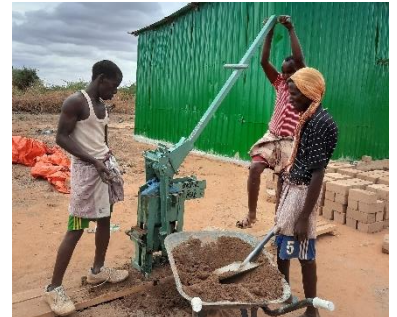
Production of CSEB with manual machine in Doolow, Jubaland – CC Enrique Sevillano Gutiérrez, CRAterre
