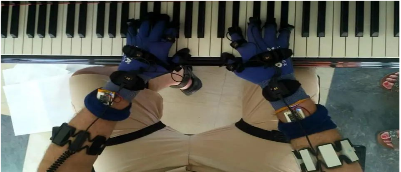
Figure 4: Flexible textile gloves for finger sensor placement
