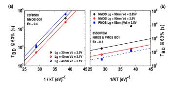
**Figure 11:** Temperature dependence of  $T_{BD}$  (63%) under Off-state stressing (a) in 28FD NFETs and (b) in 65SOI P- and N- FETs extracted from 125 °C to 25 °C. The activation energy ( $E_a$ ) remains constant for different gate channel length.
