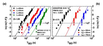
**Figure 8:** TDDB time to failure distribution for different FET gate lengths at fixed drain voltage (a) 28 FDSOI NFETs  $W = 1\mu m$  for  $V_{DS} = 2.9V$  and (b) 65 FEM PFETs  $W = 10\mu m$  for  $V_{DS} = -3.85V$ . Breakdown occurs later for longer devices (same  $\beta$  as for various  $V_{DS}$  and temperature).
