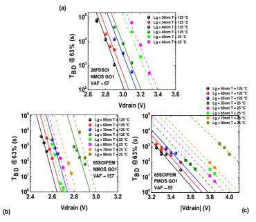
**Figure 9:**  $t_{BD}$  time to failure in GO1 28FD and 65FEM obtained at 63% vs. drain voltage with various channel length  $L_G$  in order to extract acceleration factors VAF at 125°C (solid lines) and 25°C (dash lines). (a) 28nm NFTEs, (b) 65nm NFETs and (c) 65nm PFETs. A common VAF can be extracted independently of gate channel length and temperature. VAF is found to be higher in Off-state than On-state (Table 1).
