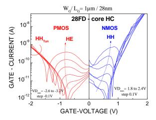
**Figure 3:** Consequence of Impact Ionization shown in NFET and PFET  $W_G$  /  $L_G = 1 \mu m$  / 28nm FDSOI under HC mode seen by gate current (Igate) measurements in thin gate-oxide for  $V_{DS}$  and  $V_{GS}$  variables, showing the distinct injection mechanisms between hot-electrons and hot-holes at low  $V_{GS}$  which turns around to a single tunneling component at high  $V_{GS}$ .
