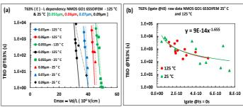
**Figure 13:** Lifetime plots defined for  $t_{BD}$  at 63% in 65nm NFET (a) vs. electrical field  $E_{max} \cong V_{DS} / L_G$  pointing out the  $L_G$  dependence between 25°C (dash lines) and 125°C (solid lines) and (b) vs. gate-oxide initial leakage current overcoming  $L_G$  dependence between 25°C and 125°.
