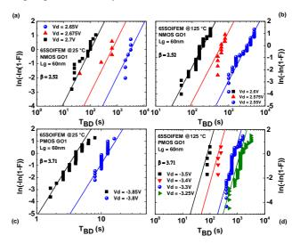
**Figure 6:** Weibit distribution plots for GO1  $W_G/L_G = 10\mu m/60nm$  65 SOI NFET and PFET at various drain voltage (a) NFET at 25 °C, (b) NFET at 125 °C, (c) PFET at 25 °C and (d) PFET at 125 °C. Weibull distribution slopes β are higher in PMOS than in NMOS an independent of bias&temperature.
