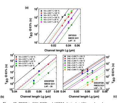
**Figure 10:** TDDB in GO1 28FD and 65FEM obtained at 63% vs. channel length  $L_G$  with various drain voltage (reverse case of **Fig. 8**) in order to extract acceleration factors LAF at 125°C (solid lines) and 25°C (dash lines). (a) 28nm NFTEs, (b) 65nm NFETs and (c) 65nm PFETs. A common LAF is extracted independently of drain bias and temperature.
