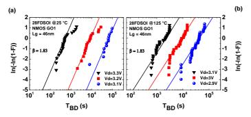
**Figure 5:** Cumulative distribution with same Weibull slope obtained in GO1  $W_G/L_G = 1\mu m/46nm$  28FDSOI NFET at various stressing drain bias between (a) 25 °C and (b) 125 °C.
