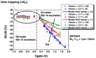
**Figure 4:**  $\Delta Id_{Lin}$  (Vd = 50 mV) in 28FDSOI N-channel  $L_G$  = 30 nm extracted at ts =  $10^4$  s. Vg dependence of  $\Delta Id_{Lin}$  under HCD in On and Off modes with Vg stress between -1 and 1.8 V with the modeling (lines) in On mode between room temperature (25 °C) and T = 125 °C.
