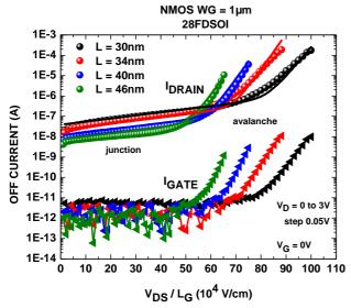
**Figure 15:**  $I_{DS}$  and  $I_{G}$  measurements and modeling at  $T=125^{\circ}C$  under Offstate ( $V_{GS}=0$ ) for  $L_{G}=30$ nm to 46nm NFETs as a function of peak lateral field approximated to  $E_{max} \approx V_{DS} / L_{G}$  showing a junction leakage and avalanche components in the diode currents. The modeling is shown in lines for  $I_{DS}$  monitoring with relatively good agreements as a function of gatelength  $L_{G}$ .
