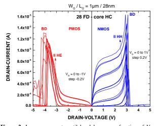
**Figure 2:**  $I_{DS}$  measurements until breakdown as a function of  $V_{DS}$  with variables  $V_{GS}$  in  $W_G$  /  $L_G$  =  $1\mu m$  / 28nm FDSOI during Off-state and subthreshold conditions. Impact ionization current is higher in NFET than in PFET under same reverse bias and BD occurs around 3V in NFET with HH injection while it seems to reach -4V with HE injection before dielectric BD in PFET.
