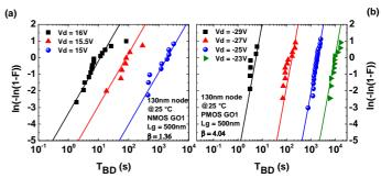
**Figure 7:** Time to breakdown distribution plots for GO1  $W_G/L_G = 10\mu m/500nm$  130nm FET at 25 °C and various drain voltage  $V_{DS}$  (a) in NMOS with lower  $\beta$  and (b) in PMOS devices.
