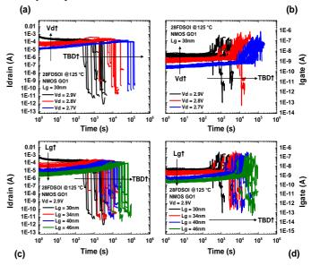
Figure 1: Leakage current until breakdown in 28nm FDSOI NFETs  $W_G = 1 \mu m$  with various  $V_{DS}$  and  $L_G$  as a function of cumulative stress time. (a) drain and (b) gate initial currents increasing with  $V_{DS}$  for  $L_G = 30 nm$ . Initial leakage current is smaller for longer devices, (c) drain current and (d) gate current monitors decreasing with  $L_G$  at the same bias  $V_{DS} = 2.9V$ .
