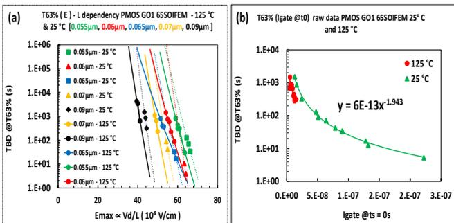
**Figure 12:** Lifetime plots as  $t_{BD}$  at 63% for 65nm PFET (a) vs. electrical field  $E_{max} \equiv V_{DS}/L_G$  enlightening  $L_G$  dependence between 25°C (dashed lines) and 125°C (solid lines) and (b) vs. gate oxide initial leakage current overcoming  $L_G$  dependence between 25°C and 125°C.
