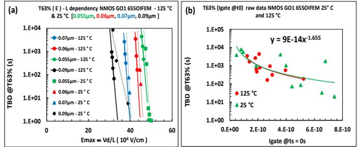
**Figure 13:** Lifetime plots defined for  $t_{BD}$  at 63% in 65nm N-FET (a) vs. electrical field  $E_{max} \equiv V_{DS}/L_G$  pointing out the  $L_G$  dependence between 25°C (dashed lines) and 125°C (solid lines) and (b) vs. gate-oxide initial leakage current overcoming  $L_G$  dependence between 25°C and 125°C.
