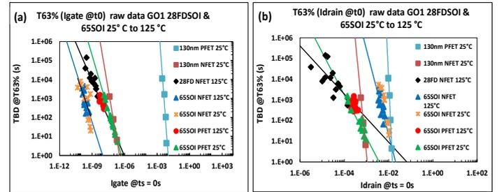
**Figure 14:**  $t_{BD}$  at 63% lifetime model as a function of initial ( $t_0$ ) leakage current in 28nm, 65nm and 130nm N- and P-FETs (a) gate current and (b) drain current monitors, between 25°C and 125°C. This shows better lifetime monitoring using gate leakage and slightly more dispersion in NFETs.
