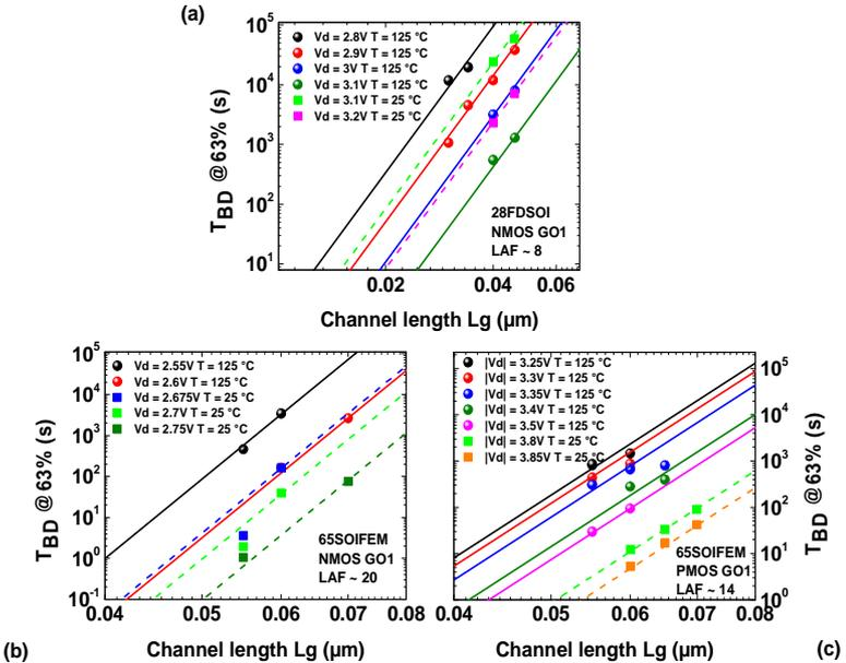
**Figure 10:** TDDB in GO1 28FD and 65FEM obtained at 63% vs. channel length  $L_G$  with various drain voltage (reverse case of **Fig. 8**) in order to extract acceleration factors LAF at 125°C (solid lines) and 25°C (dash lines). (a) 28nm NFETs, (b) 65nm NFETs and (c) 65nm PFETs. A common LAF is extracted independently of drain bias and temperature.
