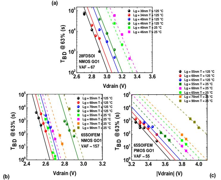
**Figure 9:**  $t_{BD}$  time to failure in GO1 28FD and 65FEM obtained at 63% vs. drain voltage with various channel length  $L_G$  in order to extract acceleration factors VAF at 125°C (solid lines) and 25°C (dash lines). (a) 28nm NFETs, (b) 65nm NFETs and (c) 65nm PFETs. A common VAF can be extracted independently of gate channel length and temperature. VAF is found to be higher in Off-state than On-state (Table 1).
