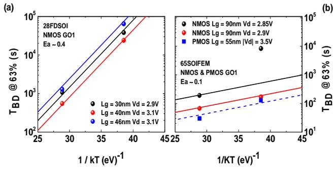
**Figure 11:** Temperature dependence of  $T_{BD}$  (63%) under Off-state stressing (a) in 28FDSOI N-FETs and (b) in 65SOI P- and N-FETs extracted from 125 °C to 25 °C. The activation energy ( $E_a$ ) remains constant for different gate channel length.
