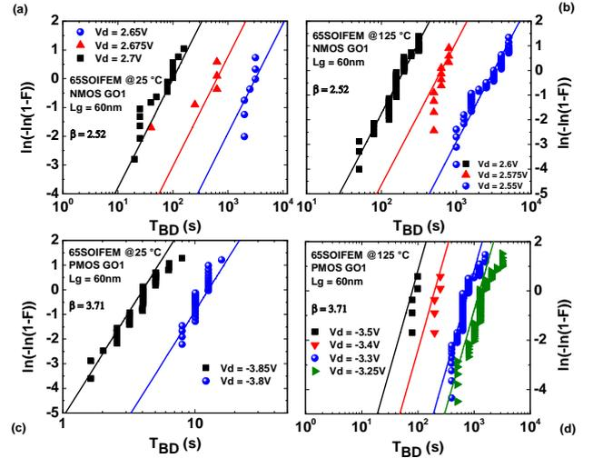
**Figure 6:** Weibit distribution plots for GO1  $W_G/L_G = 10\mu\text{m}/60\text{nm}$  65 SOI NFET and PFET at various drain voltage (a) NFET at 25 °C, (b) NFET at 125 °C, (c) PFET at 25 °C and (d) PFET at 125 °C. Weibull distribution slopes  $\beta$  are higher in PMOS than in NMOS an independent of bias&temperature.
