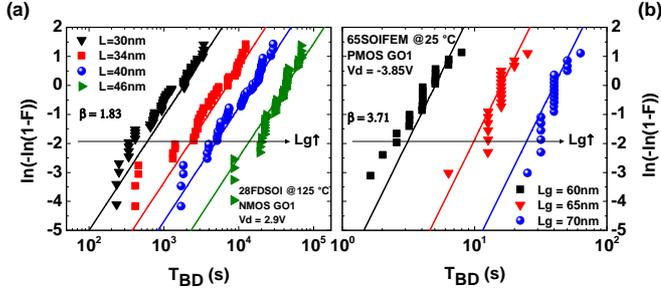
**Figure 8:** TDDB time to failure distribution for different FET gate lengths at fixed drain voltage (a) 28 FDSOI NFETs  $W = 1\mu\text{m}$  for  $V_{DS} = 2.9\text{V}$  and (b) 65 FEM PFETs  $W = 10\mu\text{m}$  for  $V_{DS} = -3.85\text{V}$ . Breakdown occurs later for longer devices (same  $\beta$  as for various  $V_{DS}$  and temperature).
