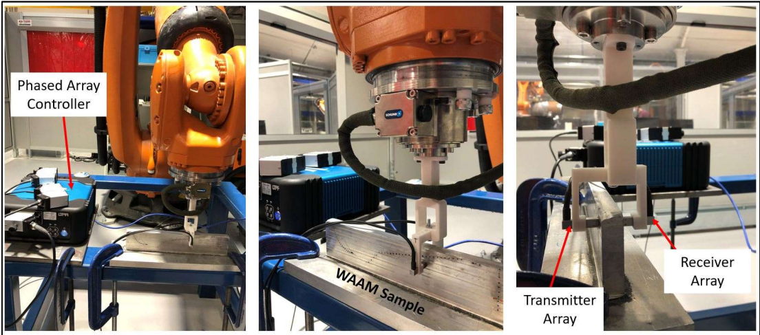
Fig. 6. PAUT system for the residual stress measurement in the WAAM sample
