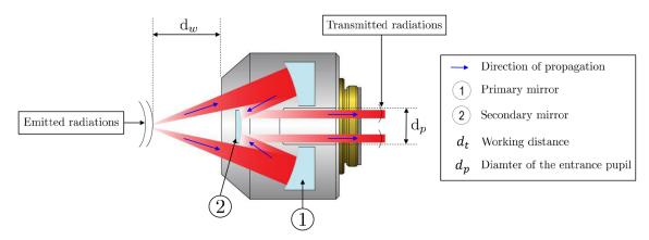
Fig. 2 Schematic illustration of the principle of transmission by double reflection of a reflective objective
