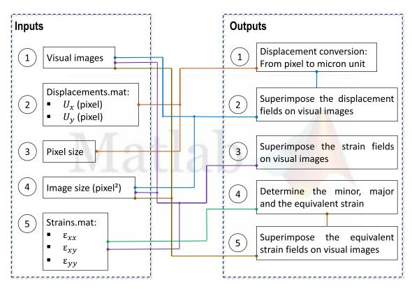
Fig. 8 Description of the developed script: inputs, outputs and links
