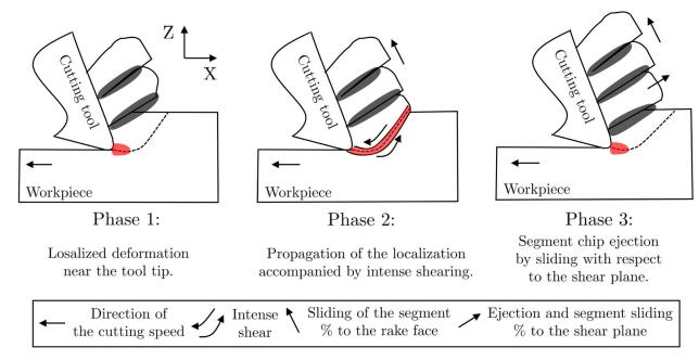
Fig. 14 Mechanisms of segmented chip formation
