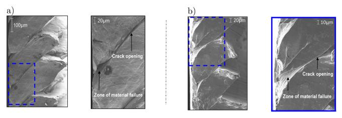
Fig. 20 SEM view on Ti-6Al-4V chip obtained during orthogonal cutting under  $V_c$ =3m/min: a)  $\gamma$ =0° and b)  $\gamma$ =15°
