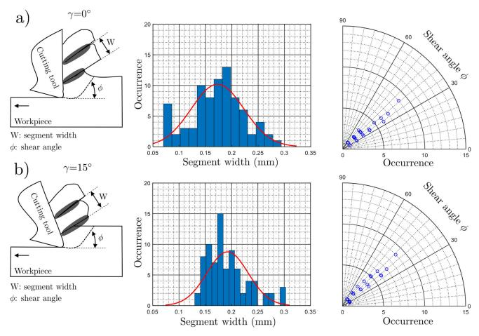
Fig. 22 Ti-6Al-4V chip characteristics: occurrence of the chip segment width and the shear angle measured from the recorded video obtained during orthogonal cutting under  $V_c$ =3m/min: a)  $\gamma$ =0° and b)  $\gamma$ =15°
