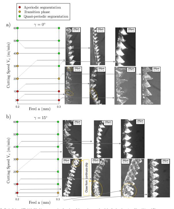
Fig. 13 Periodicity of Ti-6Al-4V chip segmentation function of the cutting speed and the feed under: a)  $\gamma$ =0° and b)  $\gamma$ =15°
