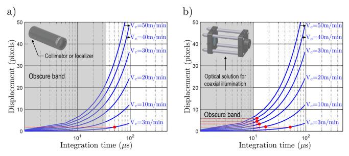
**Fig. 4** Displacement of the observed scene function of the integration time and the cutting speed: a) when using a collimator or a focalizer and b) the optical solution for coaxial illumination
