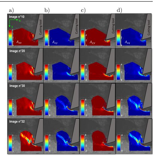
out-of-plane motion of the chip. In order to evaluate the accuracy of the measured strain fields, the effect of out-of-plane displacement was examined. An out-of-plane displacement with an increment of  $10\mu m$  was applied along the optical axis and an image was recorded at each step. The mean value of the virtual equivalent strain was measured.
