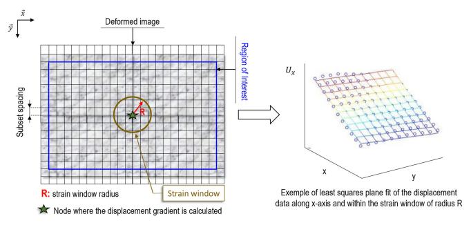
Fig. 7 Illustration of the least squares plane fit on the displacement data to determine the displacement gradient
