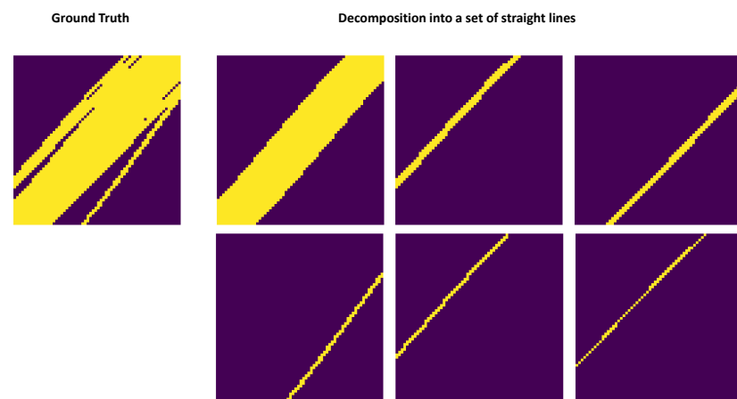
Figure 5. Result of the application of the iterative method for the decomposition of phase space into sets of straight lines. The proposed algorithm provides a minimal set of lines that when mapped in the phase space produce the same representation as the input phase space representation. Each 2D line is represented in phase space by a band with a slope and a thickness which are given by the depth and the length of the 2D line segment. Even though 2D lines are spatially disjoint in 2D space, their representation in phase space can intersect.
