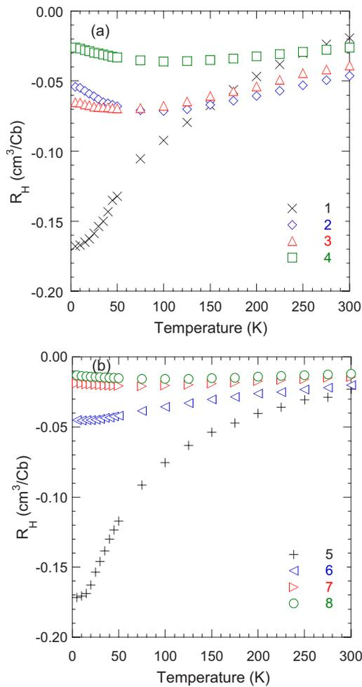
FIG. 3. (Color online) Temperature dependences of the Hall coefficient  $R_H$  for the two series of  $\text{Ca}_y\text{Co}_{4-x}\text{Ni}_x\text{Sb}_{12}$  skutterudites. (a)  $y \sim 0.10$ ; (b)  $y \sim 0.18$ . The symbols refer to the sample numbers given in Table I for the different compounds studied.
