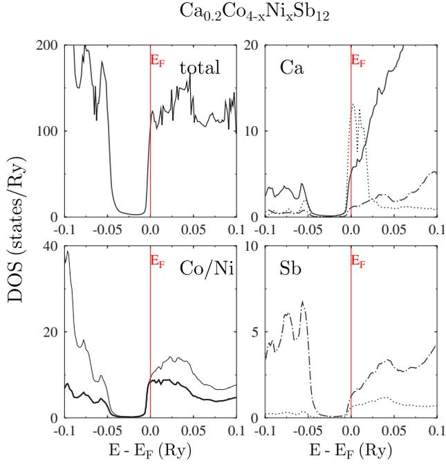
FIG. 9. (Color online) KKR-CPA density of states in  $\text{Ca}_{0.2}\text{Co}_{4-x}\text{Ni}_x\text{Sb}_{12}$  ( $x=0.04$ ). Total and  $l$ -decomposed DOS ( $s$ —dotted,  $p$ —dot-dashed,  $d$ —full lines) of constituent atoms are shown. In the case of Co (thin line) and Ni (thick line),  $s$  and  $p$  contributions are not plotted for sake of clarity.  $E_F=0$  is marked by a vertical red line.
