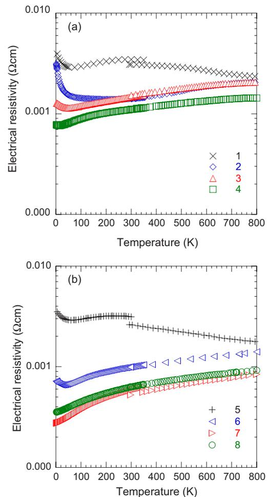
FIG. 2. (Color online) Temperature dependences of the electrical resistivity  $\rho$  for the two series of  $\text{Ca}_y\text{Co}_{4-x}\text{Ni}_x\text{Sb}_{12}$  skutterudites. (a)  $y \sim 0.10$ ; (b)  $y \sim 0.18$ . The symbols refer to the sample numbers given in Table I for the different compounds studied.
