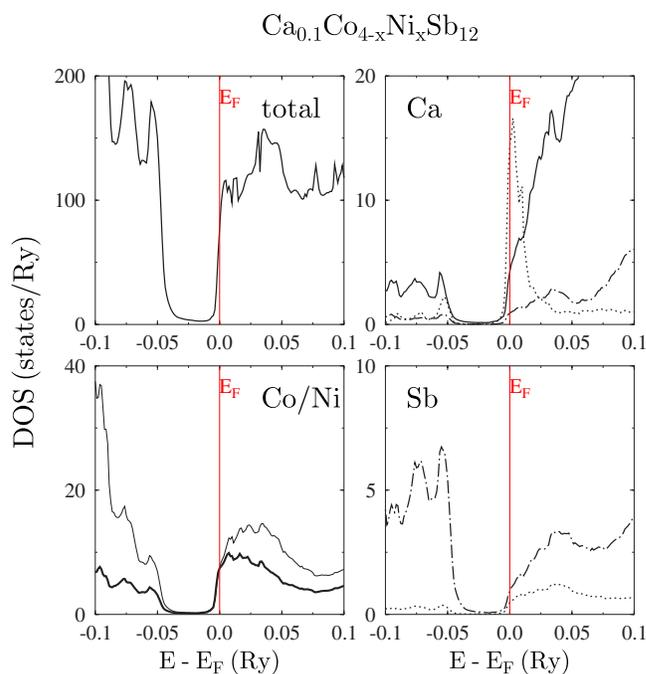
FIG. 8. (Color online) KKR-CPA density of states in  $\text{Ca}_{0.10}\text{Co}_{4-x}\text{Ni}_x\text{Sb}_{12}$  ( $x=0.04$ ). Total and  $l$ -decomposed DOS ( $s$ —dotted,  $p$ —dot-dashed,  $d$ —full lines) of constituent atoms are shown. In the case of Co (thin line) and Ni (thick line),  $s$  and  $p$  contributions are not plotted for sake of clarity.  $E_F=0$  is marked by a vertical red line.
