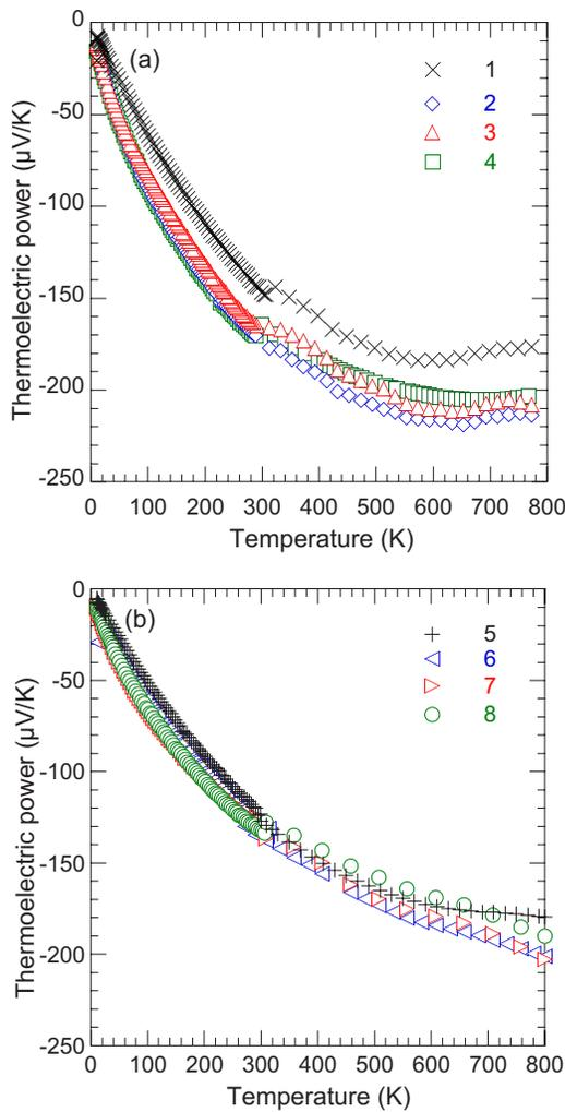
FIG. 5. (Color online) Temperature dependences of the thermoelectric power  $S$  for the two series of  $\text{Ca}_y\text{Co}_{4-x}\text{Ni}_x\text{Sb}_{12}$  skutterudites. (a)  $y \sim 0.10$ ; (b)  $y \sim 0.18$ . The symbols refer to the sample numbers given in Table I for the different compounds studied.
