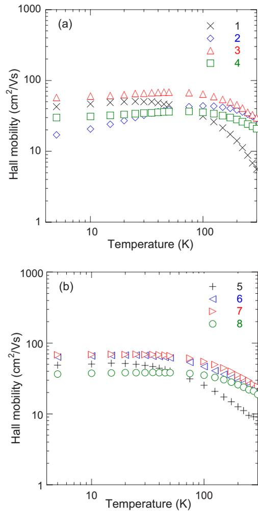
FIG. 4. (Color online) Temperature dependences of the Hall mobility  $\mu_H$  for the two series of  $\text{Ca}_y\text{Co}_{4-x}\text{Ni}_x\text{Sb}_{12}$  skutterudites. (a)  $y \sim 0.10$ ; (b)  $y \sim 0.18$ . The symbols refer to the sample numbers given in Table I for the different compounds studied.
