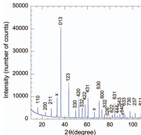
FIG. 1. (Color online) Illustrative X-ray diffraction pattern obtained for the  $\text{Ca}_y\text{Co}_{4-x}\text{Ni}_x\text{Sb}_{12}$  skutterudites. All the peaks have been indexed with regard to the JCPDS file pattern  $n^\circ 78-976$ . *x* corresponds to Si peaks (Si powder has been added to normalize the angular position of the  $\text{Ca}_y\text{Co}_{4-x}\text{Ni}_x\text{Sb}_{12}$  peaks).
