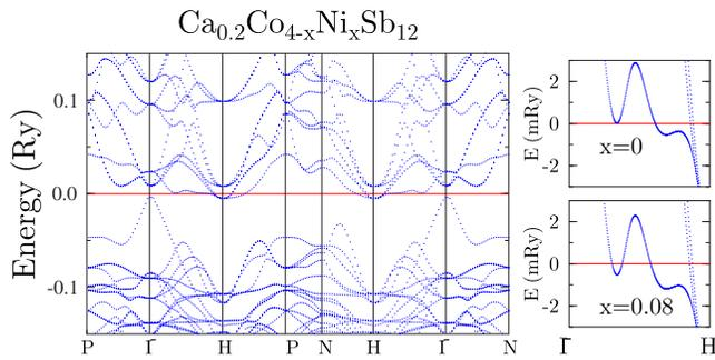
FIG. 10. (Color online) Left panel: Real part of complex energy bands  $E(k)$  in  $\text{Ca}_{0.10}\text{Co}_{4-x}\text{Ni}_x\text{Sb}_{12}$  ( $x=0.01$ ) as derived from KKR-CPA calculations.  $E_F=0$ . For sake of clarity, dispersion curves near the Fermi level are only plotted. Right panel: A flat band along the  $\Gamma$ -H direction with enlarged energy scale (mRy) and an appearance of electron-like Fermi surface pocket with Ni-doping ( $x=0$  and  $0.08$ ).
