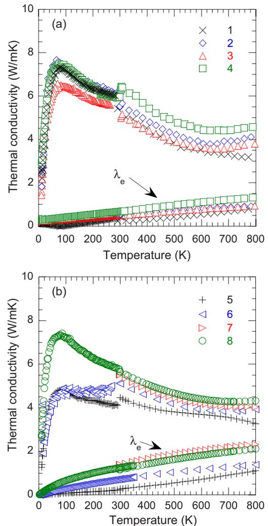
FIG. 6. (Color online) Temperature dependences of the total thermal conductivity  $\lambda$  and of the electronic thermal conductivity ( $\lambda_e$ ) for the two series of  $\text{Ca}_y\text{Co}_{4-x}\text{Ni}_x\text{Sb}_{12}$  skutterudites. (a)  $y \sim 0.10$ ; (b)  $y \sim 0.18$ . The symbols refer to the sample numbers given in Table I for the different compounds studied.
