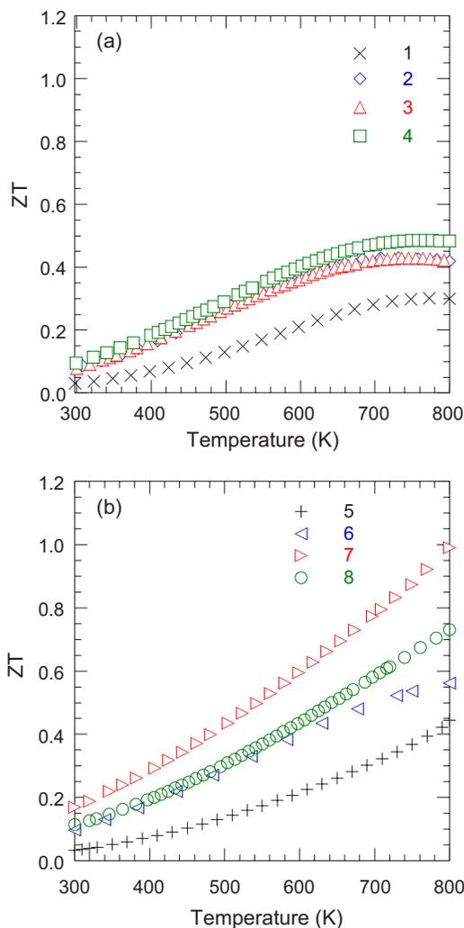
FIG. 7. (Color online) Temperature dependences of the dimensionless figure of merit  $ZT$  the two series of  $\text{Ca}_y\text{Co}_{4-x}\text{Ni}_x\text{Sb}_{12}$  skutterudites. (a)  $y \sim 0.10$ ; (b)  $y \sim 0.18$ . The symbols refer to the sample numbers given in Table I for the different compounds studied.
