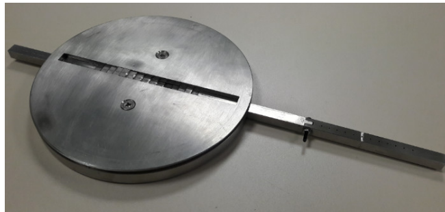
Figure 7. Dedicated calibration specimen used to calibrate the LVDT at ambient temperature and at 300 °C.
