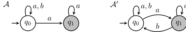
Fig. 1. Nondeterministic coBüchi automata that recognise the language of \omega -words with a finite number of b 's. A run is accepting if it eventually remains in the accepting state q_1 . \mathcal{A} is not history-deterministic as it needs to move to q_1 after the last b has been seen—information which depends on the future, rather than the history, of the input. \mathcal{A}' on the other hand is history-deterministic: to build an accepting run on any word in the language, it suffices to eventually choose, whenever the automaton is in state q_0 , the transition into q_1 .
