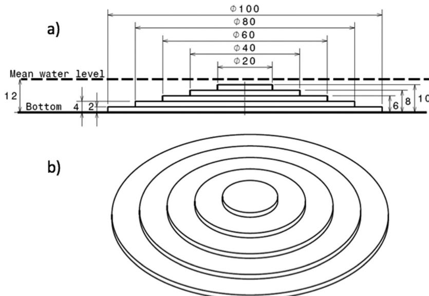
FIG. 2. Geometrical configuration C2: side view with dimensions (a) and a 3D view (b).
