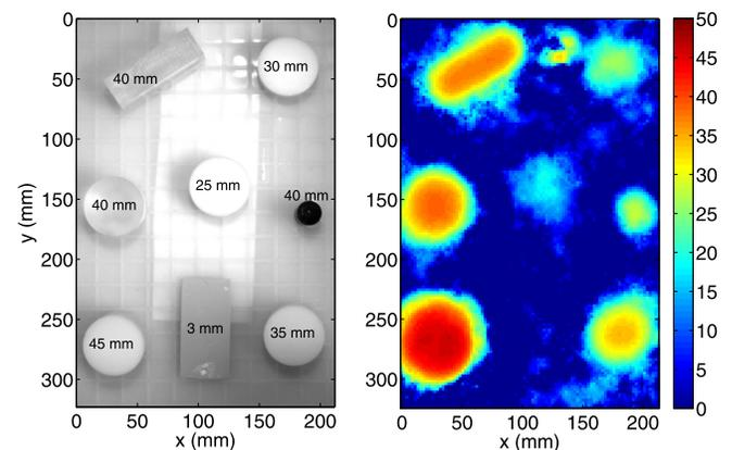
FIG. 6. Configuration C3: geometry of the bottom (left) and corresponding bathymetric maps (right) obtained experimentally by means of the circular method ( $R = 20$  mm) for liquid depth  $H_0 = 47$  mm. The color scale of the local bottom shape  $s(x,y)$  is given in millimeters.
