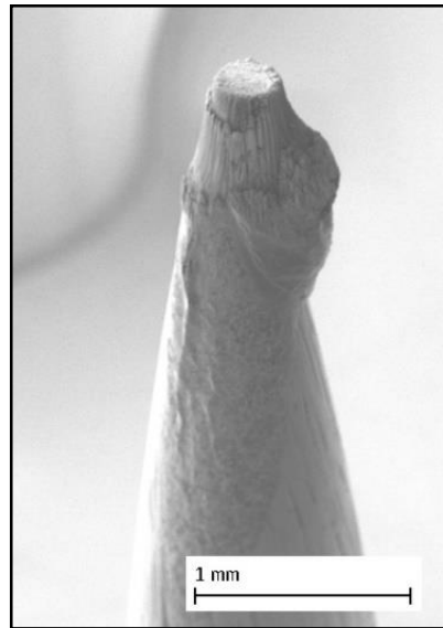
Gravure laser \varnothing = 300\mu\text{m}
