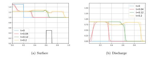
Figure 14. Travelling wave over an obstacle: surface elevation and discharge for times t = 0,0.04,0.12,0.2
