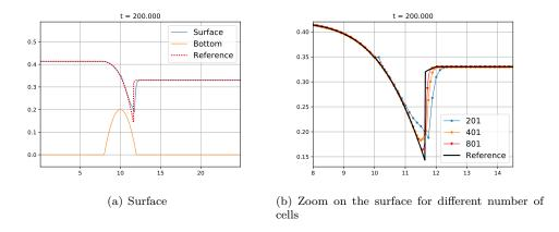
Figure 12. Transcritical steady state with shock: surface elevation
