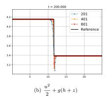
FIGURE 13. Transcritical steady state with shock: steady state condition for different number of cells
