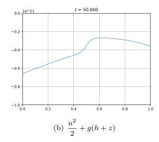
FIGURE 4. Generation of subcritical steady state from stationary initial condition: deviation from the expected constant state
