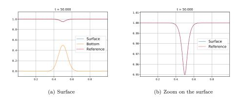
Figure 3. Generation of subcritical steady state from stationary initial condition: surface elevation compared to reference solution
