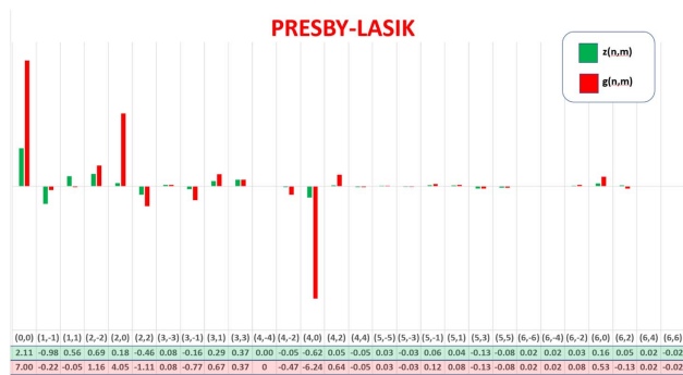
Fig. 13. Comparison between the Zernike and new expansion coefficients of an eye operated with an aspheric photoablation for hyperopia and presbyopia—PresbyLASIK.
