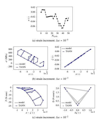
Fig. 7: Predictions of TANNs for a random loading path with strain increments varying from  $10^{-5}$  and 0.01 (beyond the training range, see Table 1): (a) loading path, (b) stress and plastic strain, (c) energy potential and dissipation rate.
