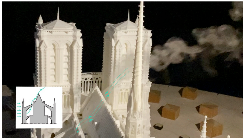
Figure 12: Flow visualization with a smoke generator in the roof region. The wind direction is perpendicular to the flank of the Cathedral ( 90^\circ ).
