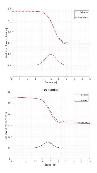
FIG. 5.4. Free surface and bed level, M = 200 cells,  $t_{end} = 16.2s$  (up) and  $t_{end} = 30s$  (bottom). Reference solution (red) and first-order weakly coupled solution (blue).
