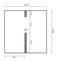
FIG. 5.8. Geometry of the dam in the squared dam break test problem.
