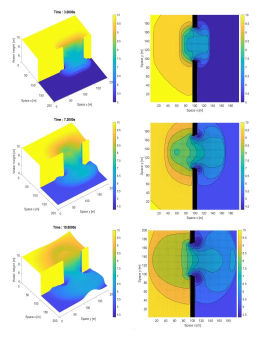
FIG. 5.9. Squared dam break; water height (left) and contour plot and velocity field (right) at time t=3.6s (up), t=7.2s (middle) and t=10.8s (bottom). Dam in black. 2D extension of second order scheme with M=100 cells and CFL=0.25.
