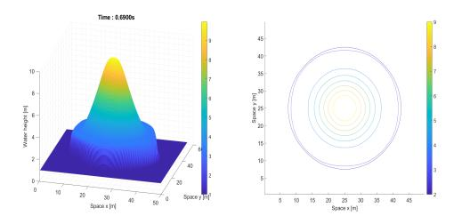
FIG. 5.6. 2D circular dam break on wet bed; water height (left) and its contour plot (right). 2D extension of first-order scheme solution. M = 100 cells,  $t_{End} = 0.69s$  and CFL = 0.45.
