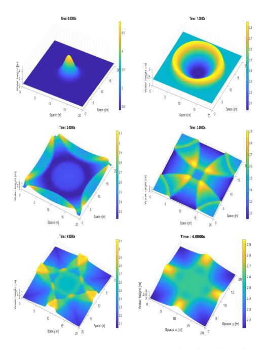
FIG. 5.7. Water drop in a basin; water height at time t=0s (up, left), t=1s (up, right), t=2s (middle, left), t=3s (middle, right) and t=4s (bottom). M=100 cells, CFL=0.25 and CFL=0.45 for the 2D extension of second and first order scheme respectively. 2D-extension of the 1D first-order scheme used only in the image on the bottom-right.
